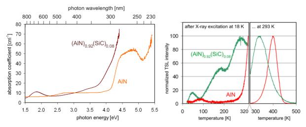
Fig. 2: Comparison of properties between AlN and (AlN)<sub>0.92</sub>(SiC)<sub>0.08</sub> bulk crystals. a) Optical absorption in the visible and UV wavelength range. b) Thermally stimulated panchromatic luminescence after X-ray excitation at 18 K and 293 K.
