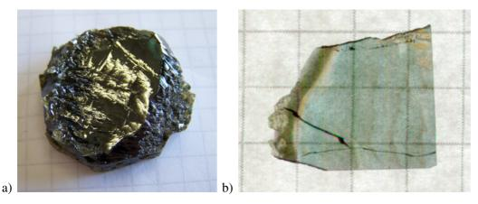
Fig. 1: a) Photograph (on 5 mm grid) of a  $(AlN)_{0,92}(SiC)_{0,08}$  bulk crystal; b) photograph of a 410 µm mm thick wafer cut from this crystal (on 5 mm grid).
